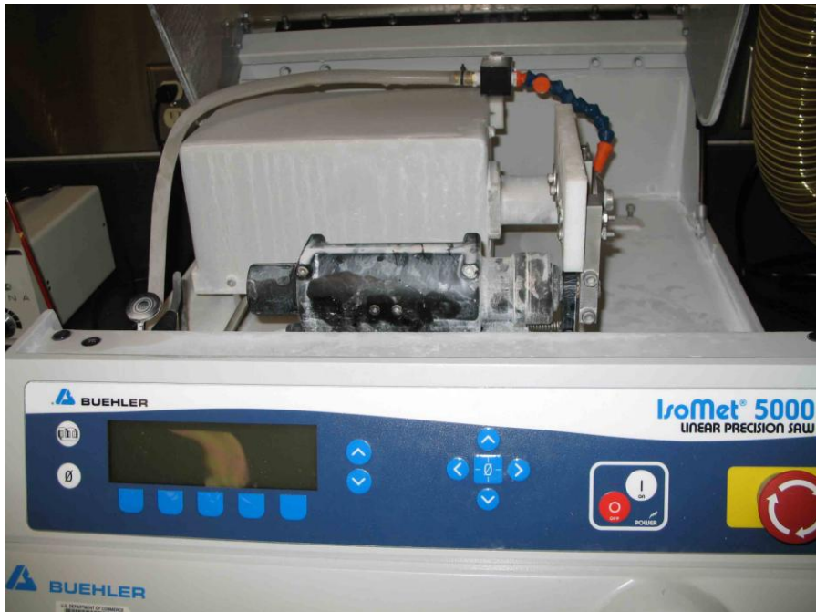
Figure 3. Close up of AFSC's new Isomet 5000 saw used to produce otolith thin sections.
